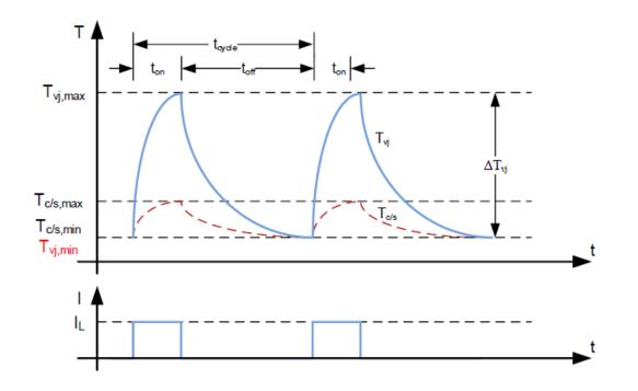
Figure 9.1: Example for current and temperature curve PC<sub>sec</sub>
