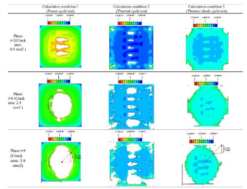
Figure 24. Crack propagation on solder between copper plate and silicon plate (creep contour).
