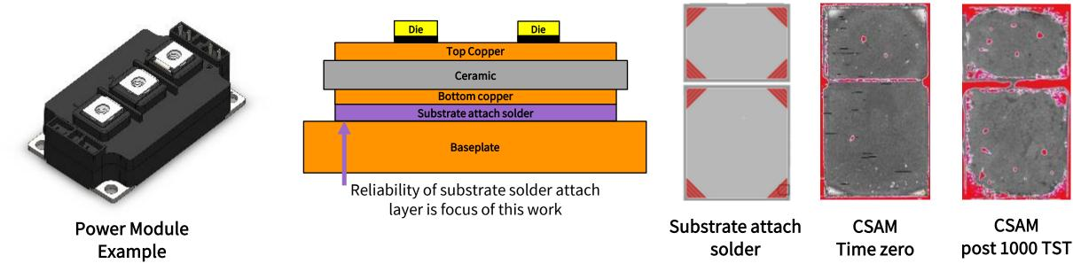
**Motivation**: Number of Thermal Shock cycles to failure (N<sub>f</sub>) analysis of power module substrate attach layer
