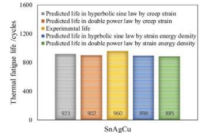
Fig. 19 – Comparison of thermo-mechanical fatigue lives from the FEM simulation and the test.
