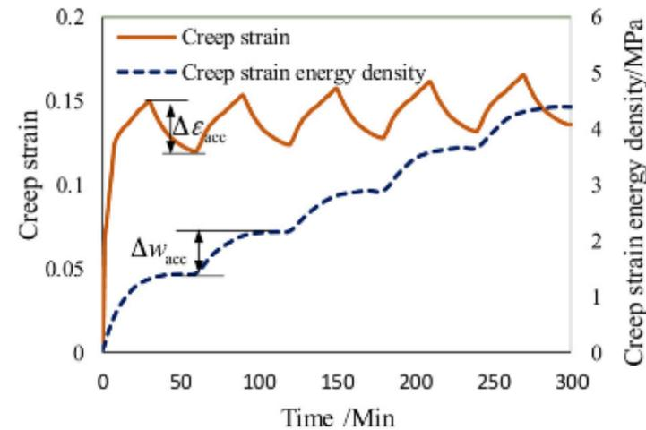
Fig. 17 – Creep strain and creep strain energy density with temperature cycles.
