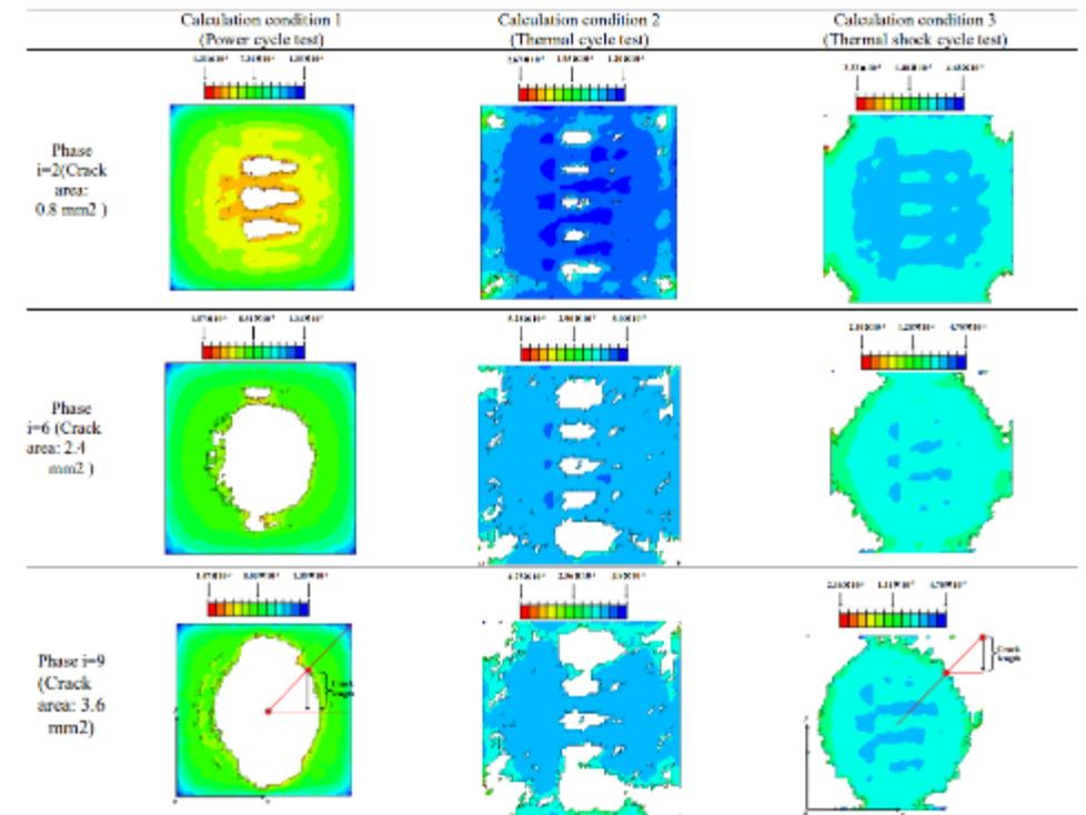
Figure 24. Crack propagation on solder between copper plate and silicon plate (creep contour).
