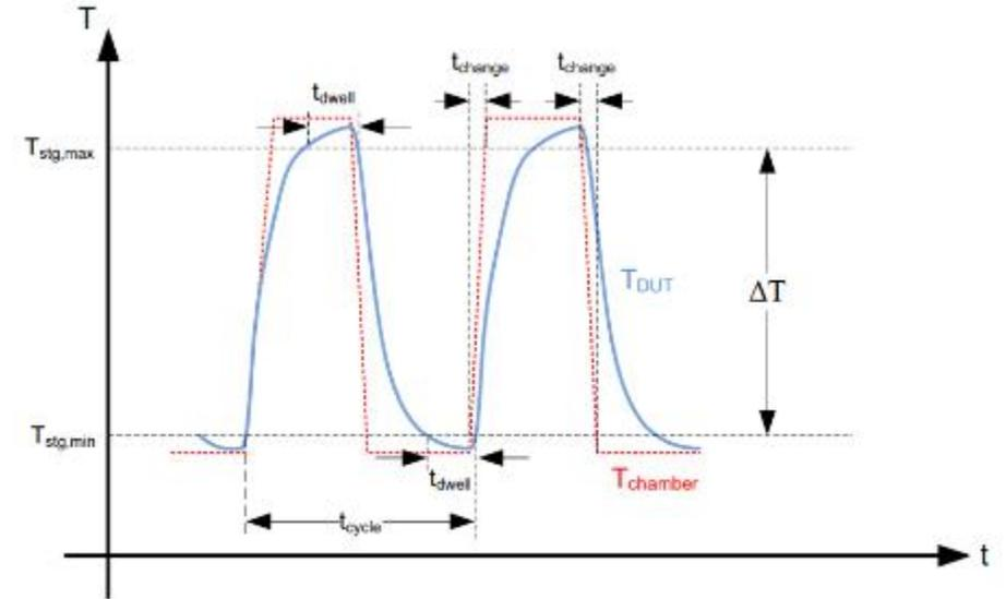
Figure 8.1: Example for TST temperature curve
