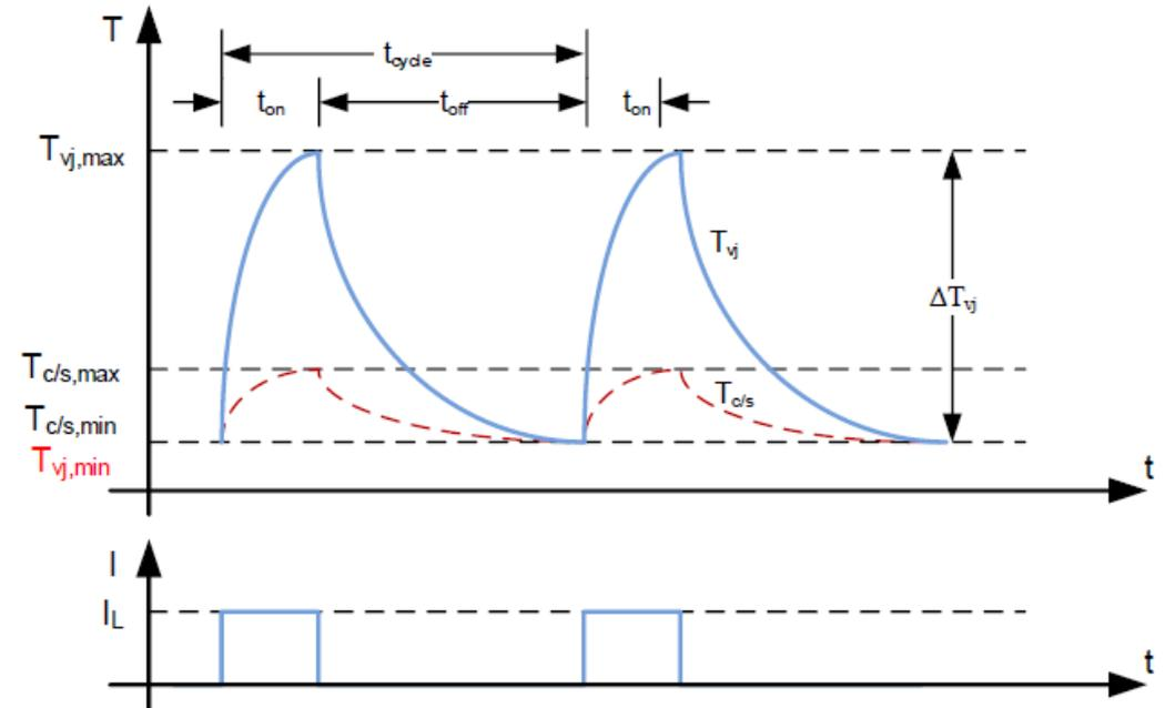
Figure 9.1: Example for current and temperature curve  $PC_{sec}$
