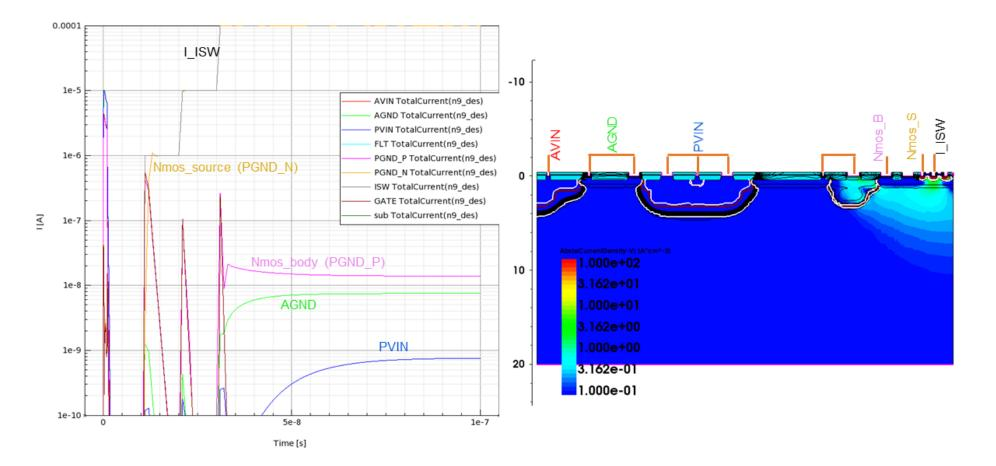
Current vs time waveforms for all terminals. Notice I\_ISW and NMOS\_source waveforms are overlapping at most of the time. Structure cross-section view of electron current density color map & static potential contours with -1V~1V range, at 100ns time point.
