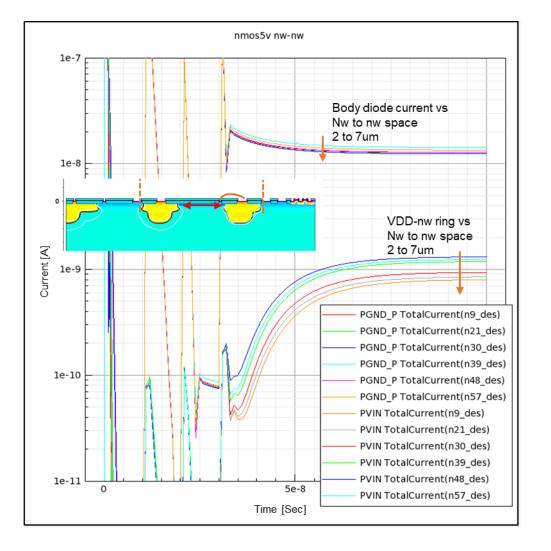
Current vs time waveforms responses to NW to NW distance variations, from 2  $\mu$ m to 7  $\mu$ m, step by 1  $\mu$ m. Vertical axis is zoomed in to focus on body diode and VDD-nw ring currents.
