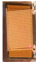
Microtransformer (1.7mm x 4.0mm)
