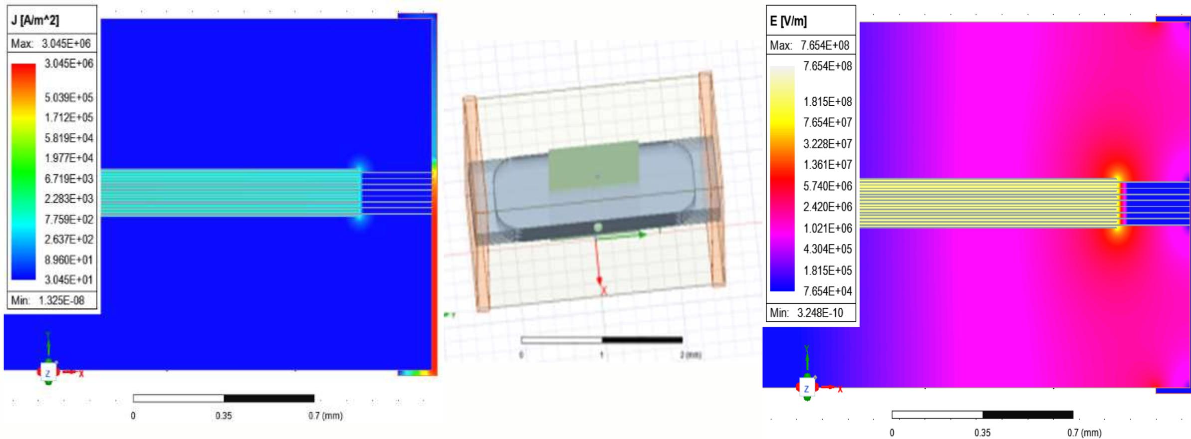
ANSYS® Maxwell® 3D Model Cut plane in center for 2D current density and electric field plots
