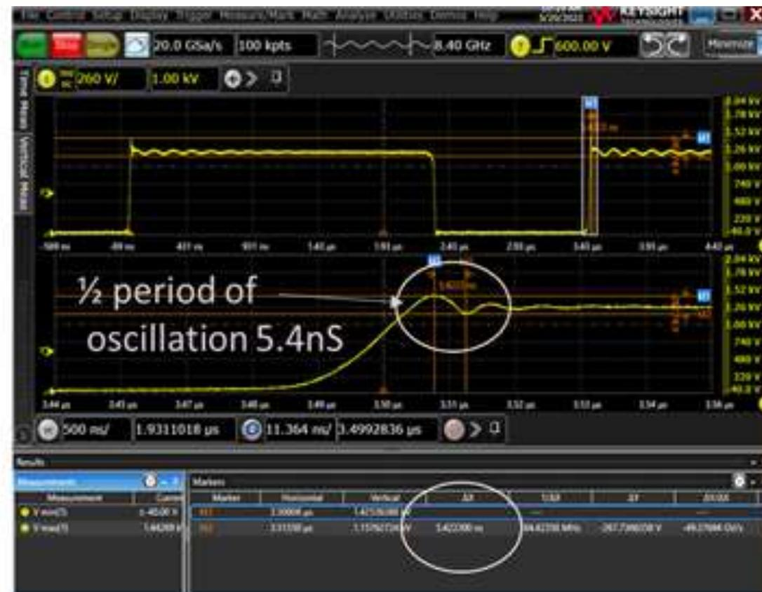
dV/dt of 70 V/ns,  $V_{\text{overshoot}}$  of 1.47 kV, and loop resonant frequency of approximately 580 MHz.
