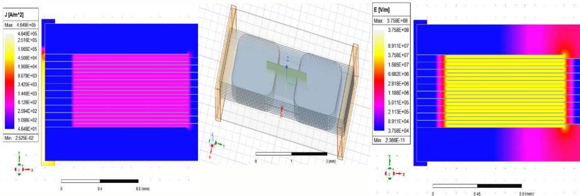
ANSYS® Maxwell® 3D Model Cut plane in center for 2D current density and electric field plots
