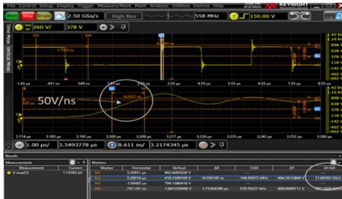
dV/dt across MLCC in chamber at 25 C measured with differential probe ~ 50V/ns .
